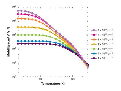
Electron mobilities as a function of carrier density for La-doped SrTiO<sub>3</sub> films grown by molecular beam epitaxy. Reprinted with permission from Reference 93. Copyright 2013, American Institute of Physics.
