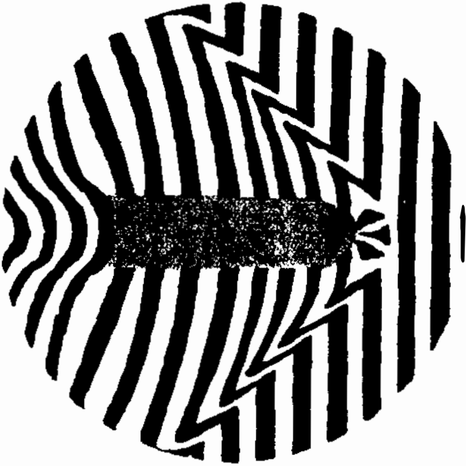
Figure 19 Interferogram of flow field around a supersonic projectile (Mach 1923).
