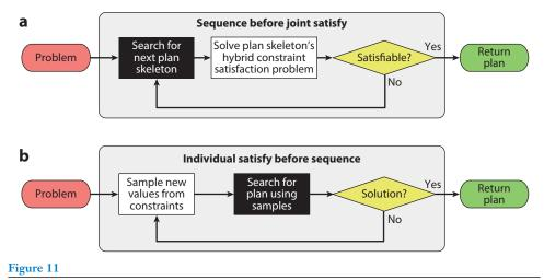
Flowcharts for two representative task and motion planning algorithms. (*a*) An algorithm that iteratively searches in the space of unbound plans and jointly satisfies the set of constraints (Section 3.3.1). (*b*) An algorithm that iteratively performs individual sampling before searching in the space of fully bound plans (Section 3.3.2).
