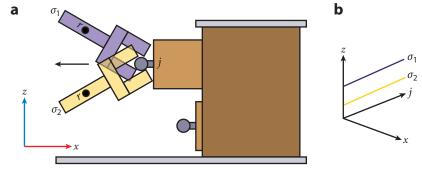
Constrained motion planning for a system in which a gripper pulls a drawer. (*a*) The gripper and the drawer. The pose of the gripper relative to the drawer handle induces the 1D mode constraints  $\sigma_1$  and  $\sigma_2$ . (*b*) The combined configuration space and the feasible spaces  $W_{F_{\sigma_1}}$  and  $W_{F_{\sigma_2}}$  (*lines*). The modes  $\sigma_1$  and  $\sigma_2$  allow the gripper to move along different 1D lines in this 3D space, depending on the grasp of the drawer handle.
