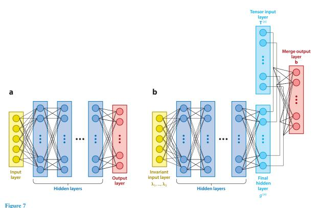
Comparison of standard neural network architecture (a) with modified neural network for identifying Galilean invariant Reynolds stress models (b). Abbreviations: **b**, anisotropy tensor;  $g^{(n)}$ , scalar coefficients weighing the basis tensors;  $\mathbf{T}^{(n)}$ , isotropic basis tensors;  $\lambda_1, \ldots, \lambda_5$ , five tensor invariants. Figure adapted with permission from Ling et al. (2016b).
