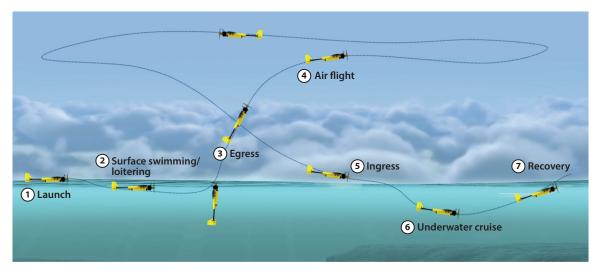
An overview of the operation of a cross-domain unoccupied aircraft system that can conduct aerial operations, land on the water for surface operations, and then submerge for underwater operations. Image courtesy of M. Andersen, Teledyne Scientific.
