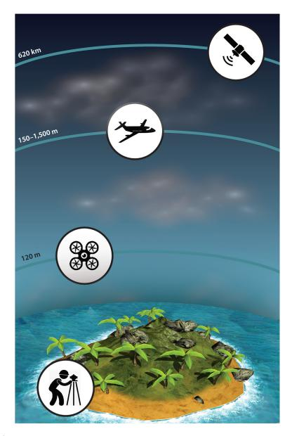
An overview of how unoccupied aircraft systems fit into the sampling spectrum. Marine scientists and resource managers can collect high-resolution data at ground level but cannot efficiently sample larger spaces. Previously, collecting data quickly over larger scales required the use of occupied aircraft or satellites in orbit, both of which are constrained by atmospheric effects and present logistical challenges.
