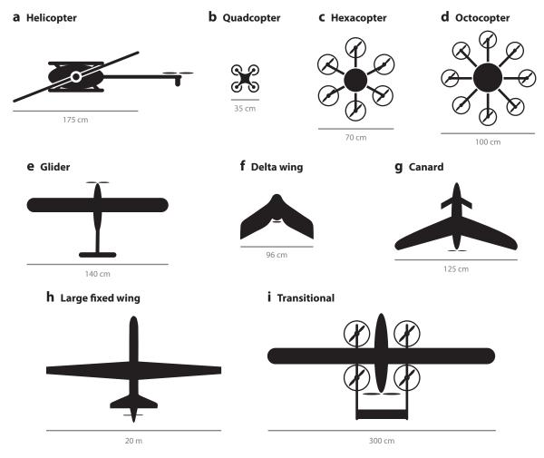
Plan views of typical (*a*–*d*) multirotor, (*e*–*b*) fixed-wing, and (*i*) transitional unoccupied aircraft systems used in marine science and conservation, along with representative wingspans.
