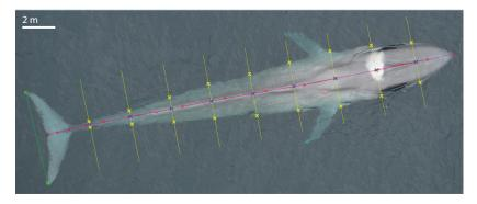
An aerial image of a blue whale generated from a photogrammetric survey using an unoccupied aircraft system. The whale has been proportioned into tenths, and measurements of its width are represented by yellow lines perpendicular to the long axis of the whale.
