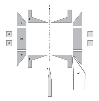
Simplified diagram of the Harvard cylindrical Penning trap (not to scale) (80, 81). Abbreviations: *E*, end-cap electrodes; *C*, compensation electrodes; *RE*, ring electrodes; *R*, nickel rings for generating magnetic field gradient; *F*, field emission point used to generate electrons; *M*, microwave input.
